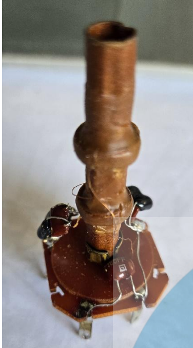
Figure 13 - Discrete capacitors installed
