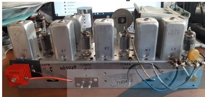
Figure 21 - Chassis rear view - note handwritten markings by various technicians, as well as factory stamps
