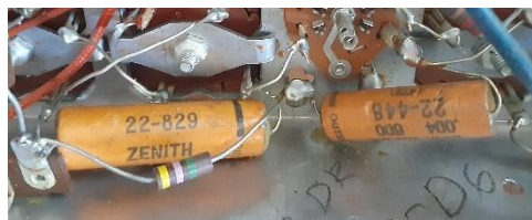
Figure 13 - Wax-and-paper capacitors with "outside foil end" marked
