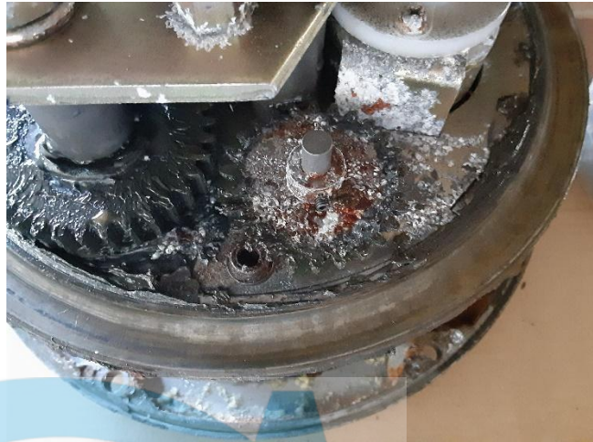
Figure 3 - Condition of potentiometer drive gear
