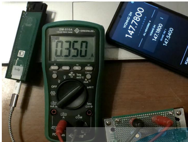
Figure 15 - Receive current draw
