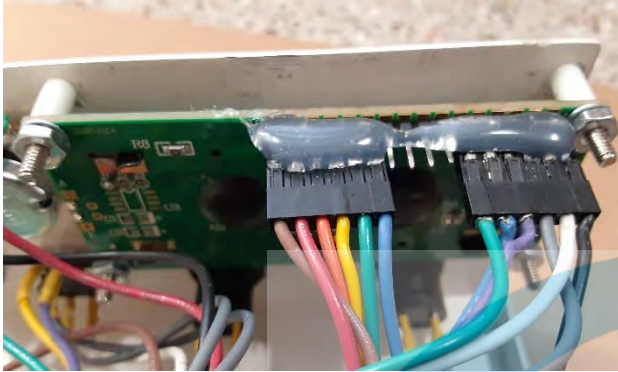
Figure 15 - Hot-glued wiring connectors
