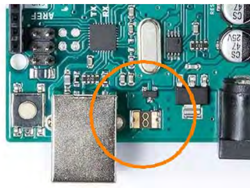
Figure 7 - Arduino fuse to be removed
