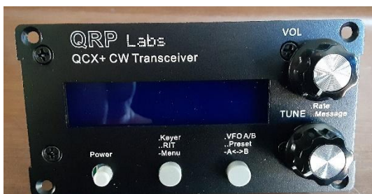
Figure 9 - Front panel assembled
