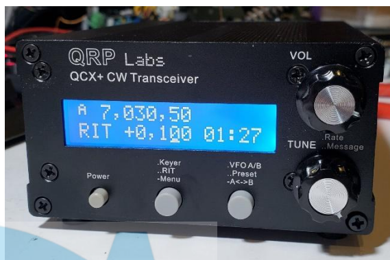
Figure 1 - QRP Labs QCX+ 5W transceiver
