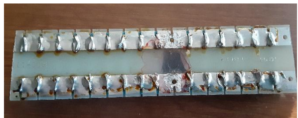
Figure 3 - PCB with resistors removed
