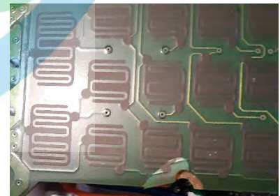
Figure 3 - Torn PCB traces
