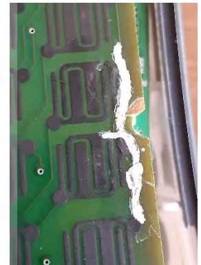
Figure 5 - Ink applied to PCB
