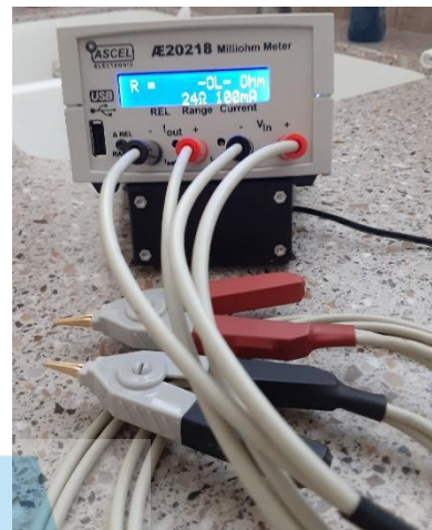
Figure 1 - Kelvin test lead set
