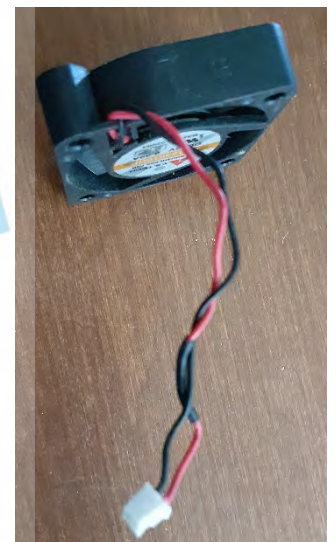
Figure 6 - Repaired fan wire
