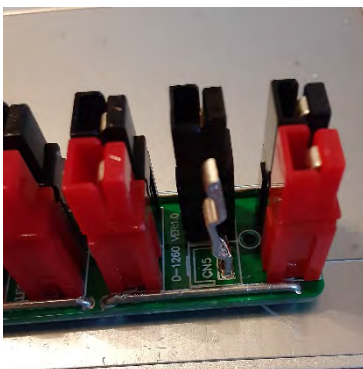
Figure 6 - Connector shell removed
