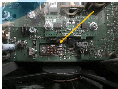
Figure 5 - Heatsink on pre-driver transistor
