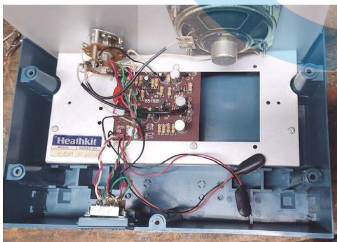
Figure 4 - IT-5283 interior, showing mounted PCB
