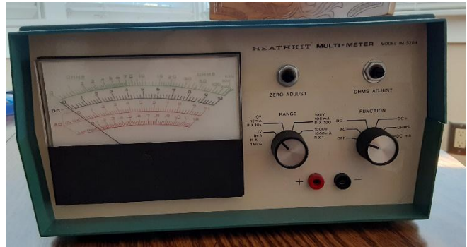
Figure 1 - Heathkit® IM-5284 multimeter as refurbished
