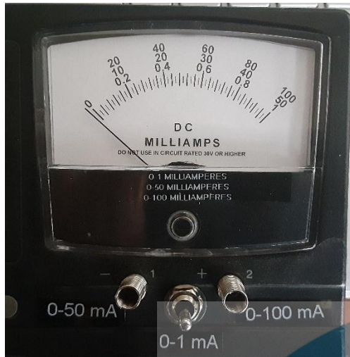
Figure 10 - Modified ammeter on panel
