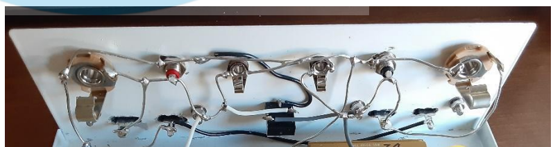
Figure 4 - Rear panel wiring in place
