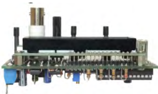
Figure 10 - LCD panel installed
