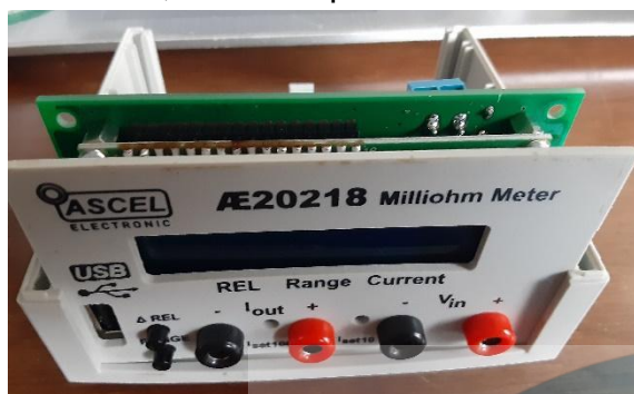
Figure 8 - Front panel and PCB installed
