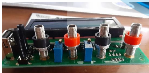
Figure 7 - Banana jacks ready for panel
